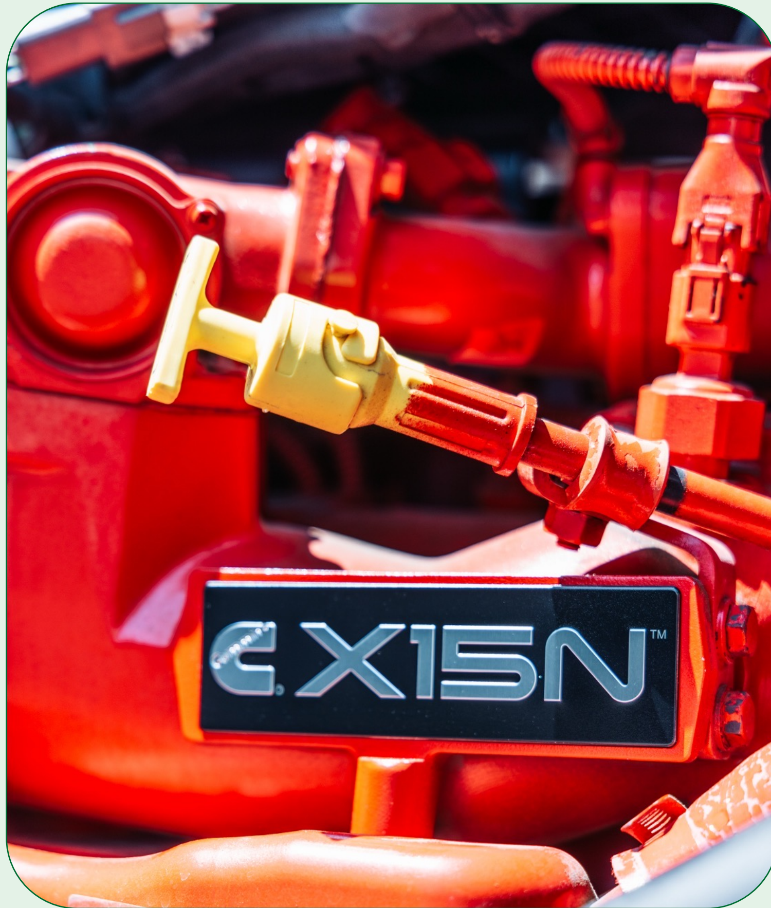
15-liter big bore natural gas engine made by Cummins
